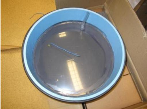
*vii.* Cut inner rubber tube into approximately 3 in. straps and stretch the strap around PVC lid. Secure the rubber strap with super glue to ensure airtight seal. This rubber strap will be used to close the chamber during headspace gas sampling.
